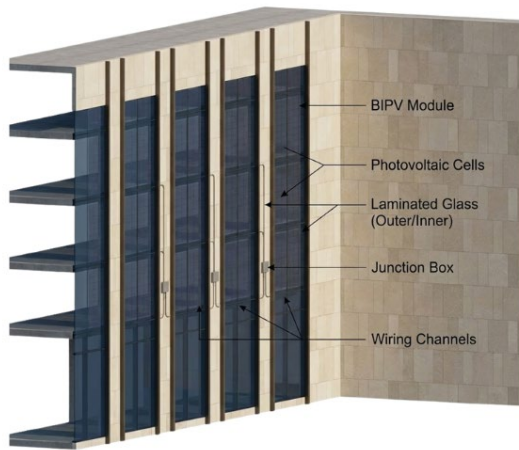
Wall Section: BIPV System
